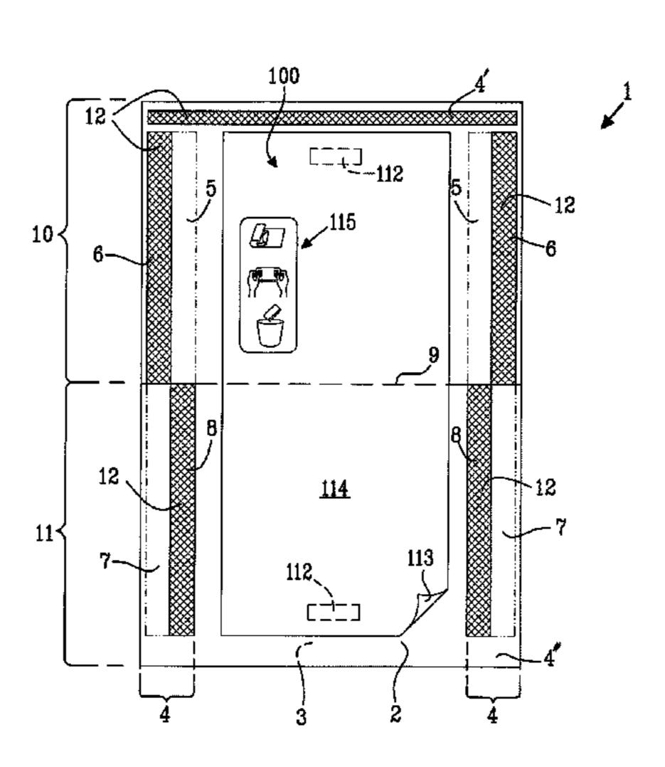
wrap. The user prompting device is arranged to prompt the user to employ the second disposal function of the packaging unit.
