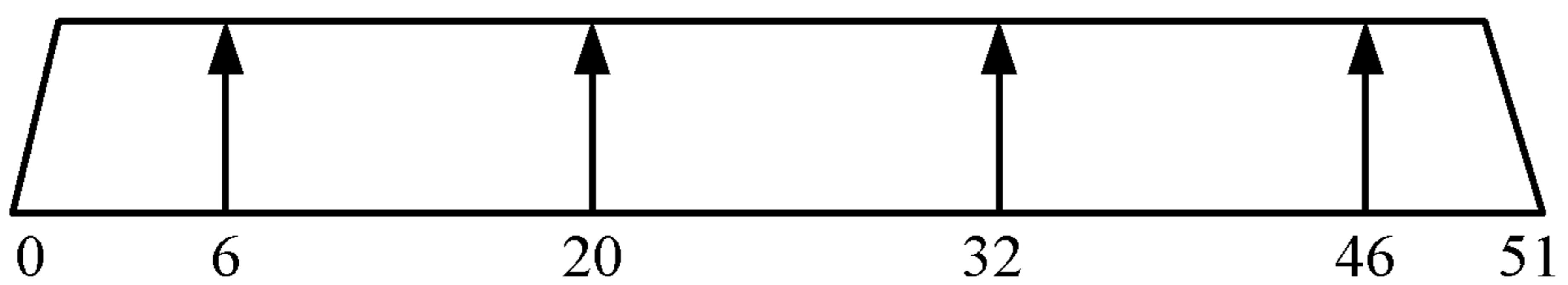
11a 52-tone pilot structure with aligning to pilots in 26-tone RU
