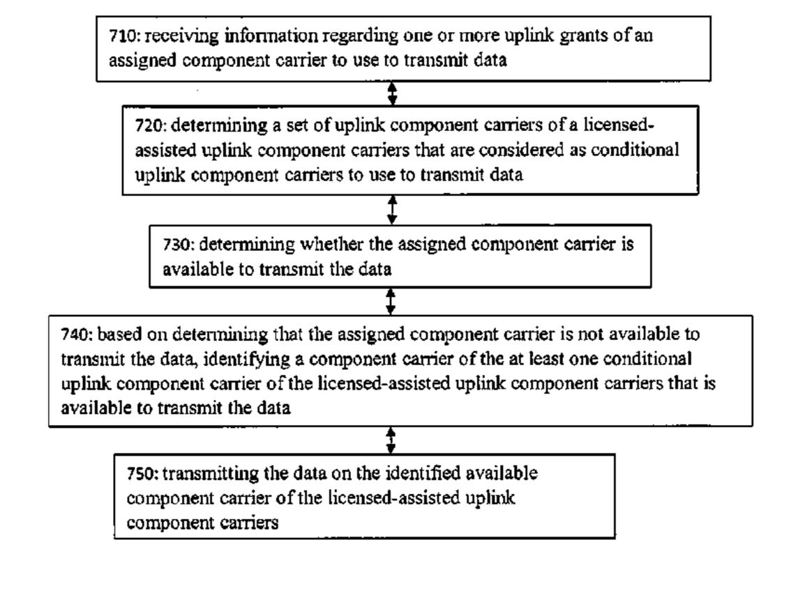
data; and transmitting the data on the identified available component carrier of the licensed-assisted uplink component carriers, is disclosed.
