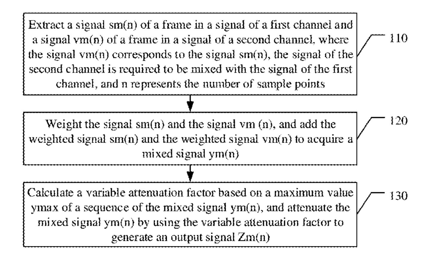
mixed signal ym(n) by using the variable attenuation factor to generate an output signal Zm(n).
