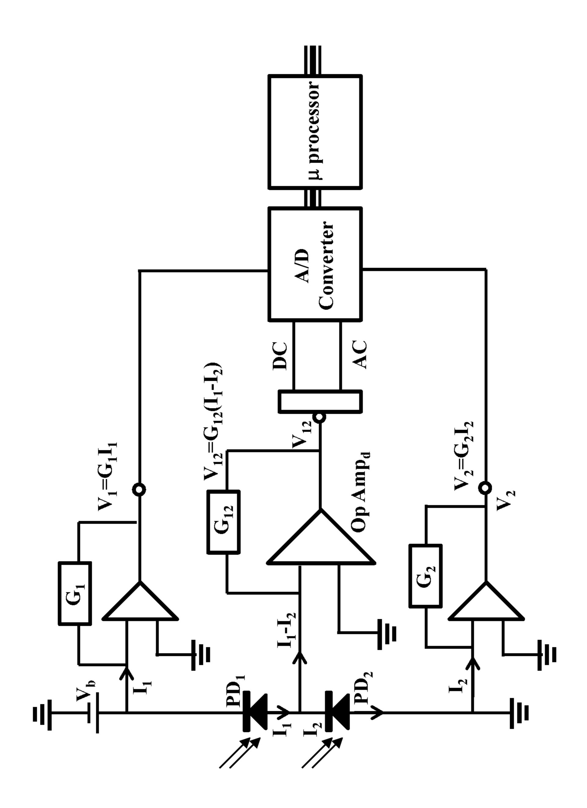
IG. 3 Illustration of detection with balanced detection circuitry
