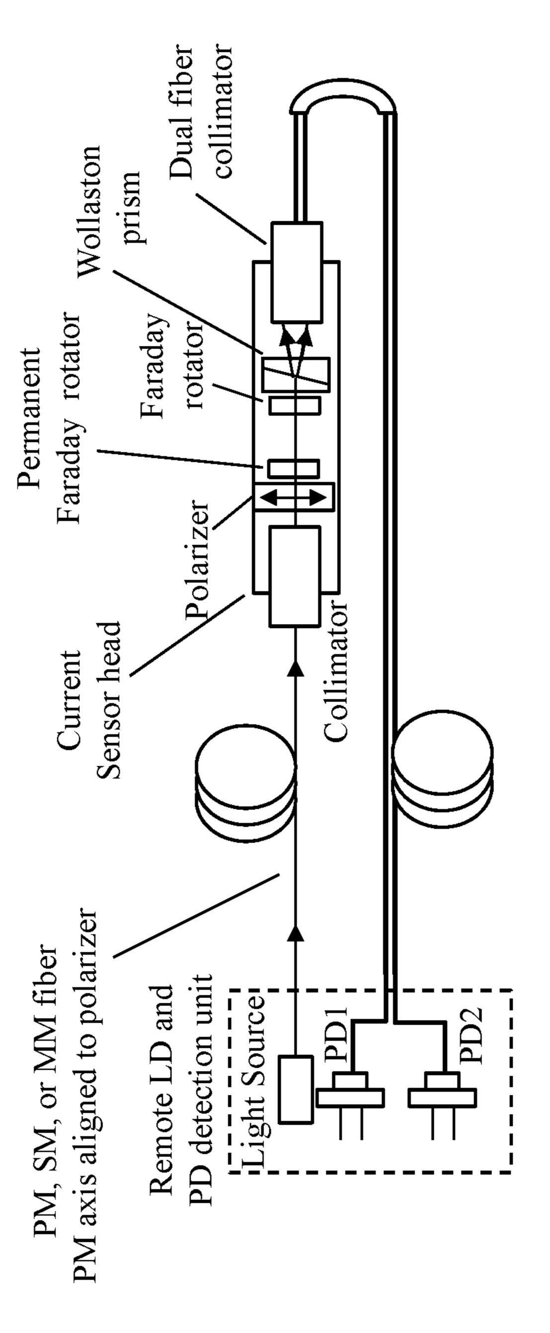
Illustration of a transmissive current sensor
