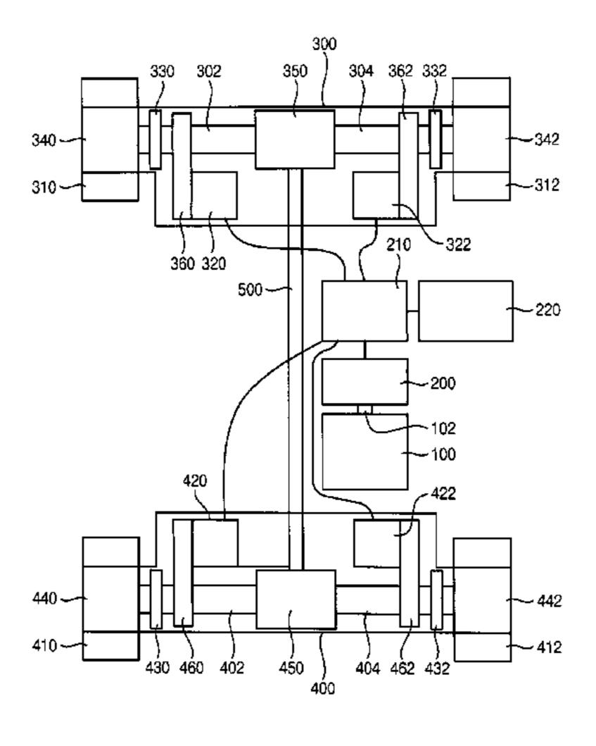
unit operatively connected to the front drive shaft and the rear drive shaft and configured to transmit the conversion torque between the front axle and the rear axle.
