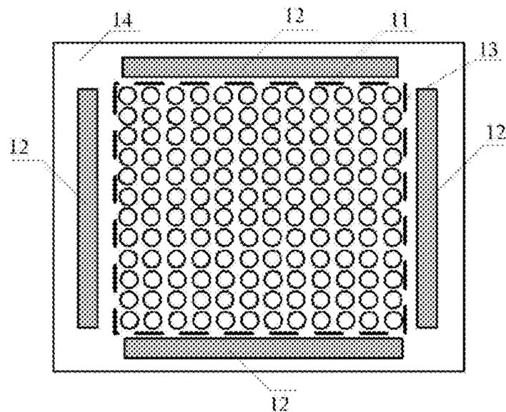
being used for eliminating or reducing droplets at positions corresponding to the edge area where the droplet removing component is located.
