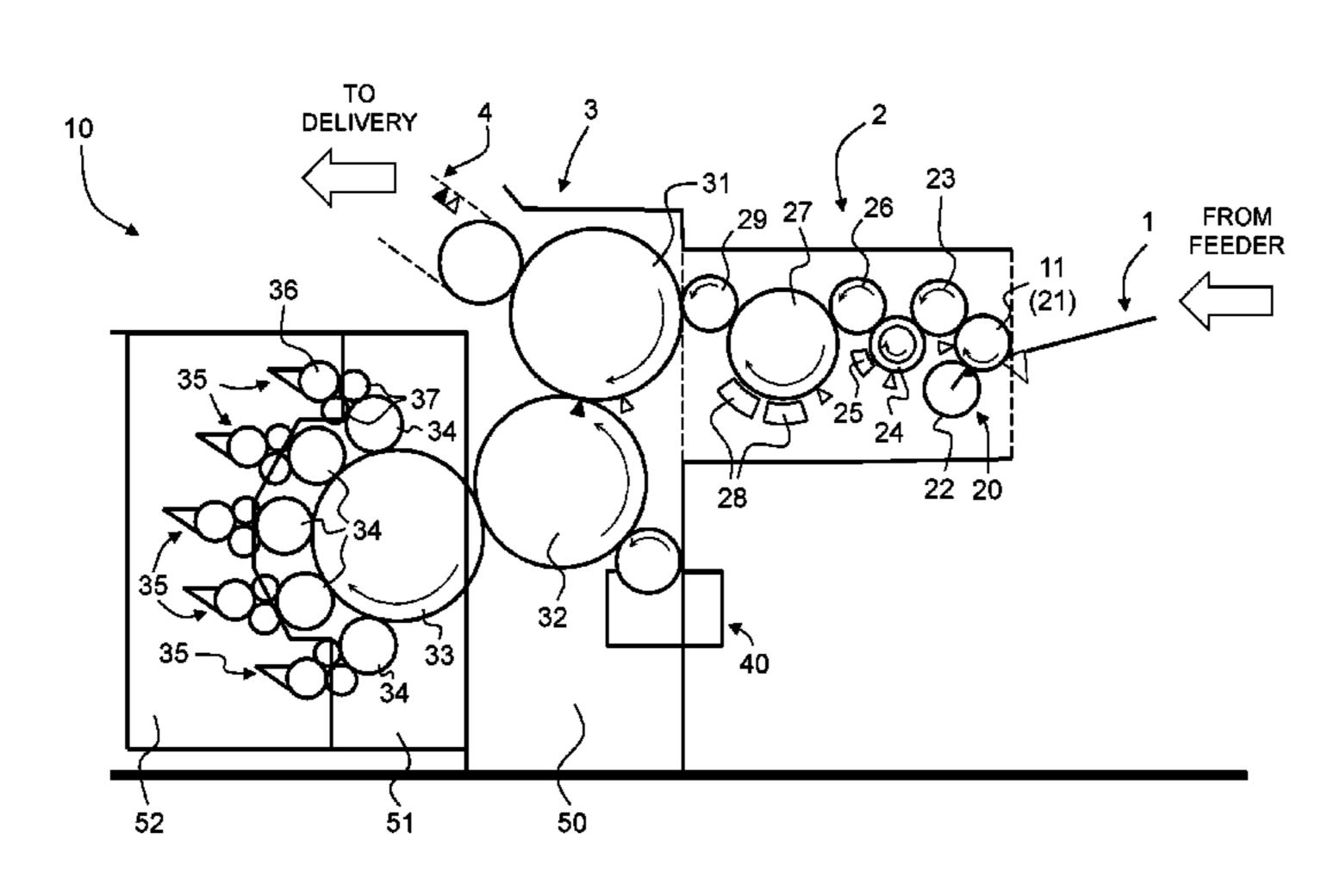
which magnetic unit is designed to magnetically induce an optically-variable effect in the pattern of optically-variable ink applied by the screen printing unit (20; 20\*). The screen printing group (2; 2\*) further comprises at least one drying/ curing unit (25, 28; 25\*, 28\*) designed to dry/cure the pattern of optically-variable ink in which the opticallyvariable effect has been induced by the magnetic unit (24), prior to transfer of the substrates to the intaglio printing group (**3**).
