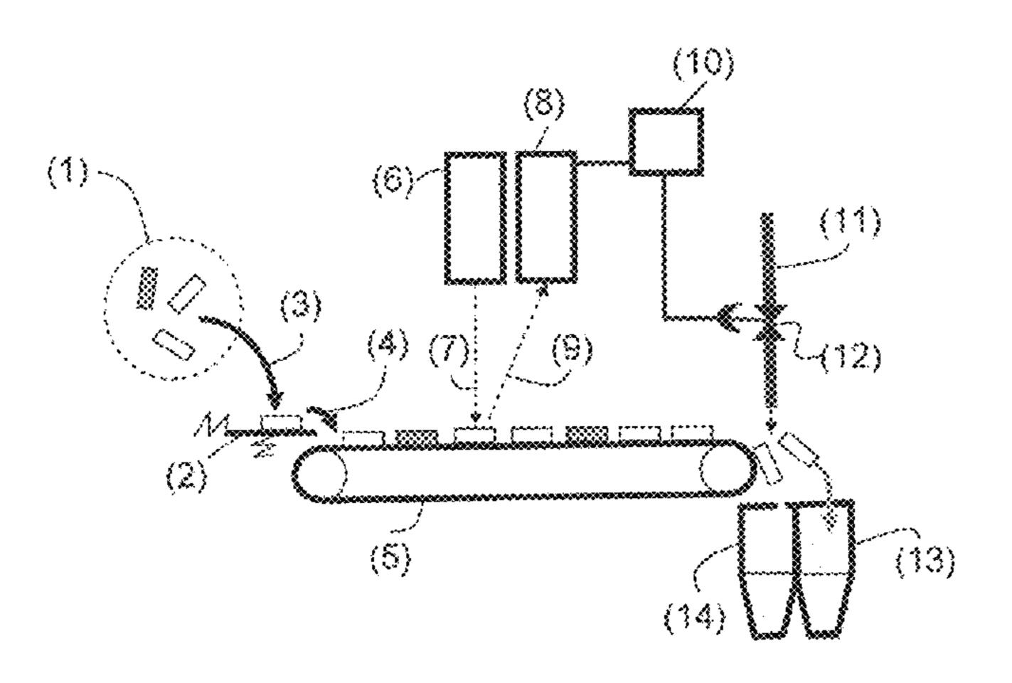
the contaminant content, starting from a sorting threshold that corresponds to a content and that is defined by the operator.
