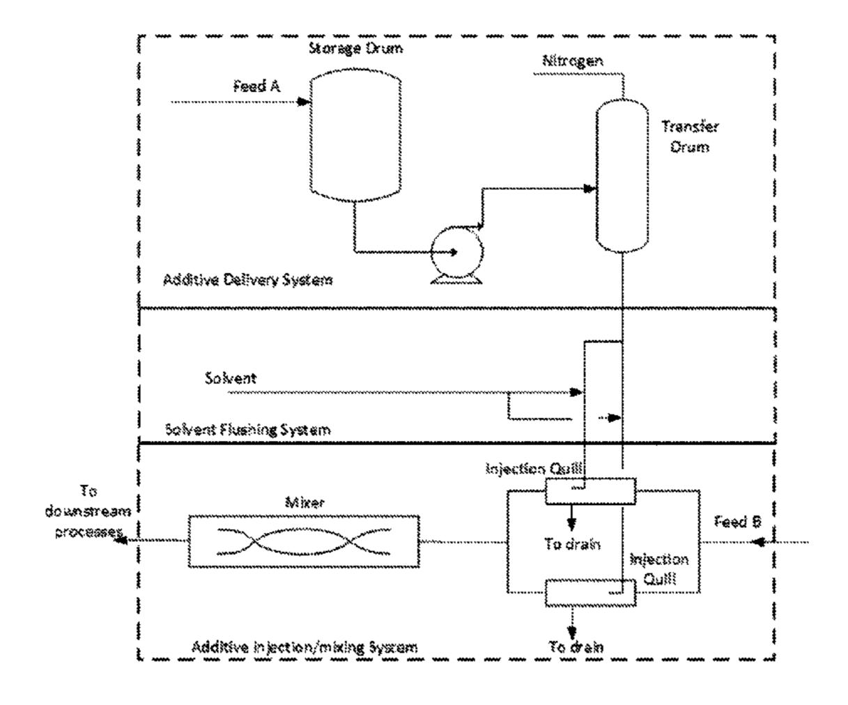
c. injecting the immiscible liquid stream into the larger liquid stream in an additive injection and mixing system comprising injection quills.
