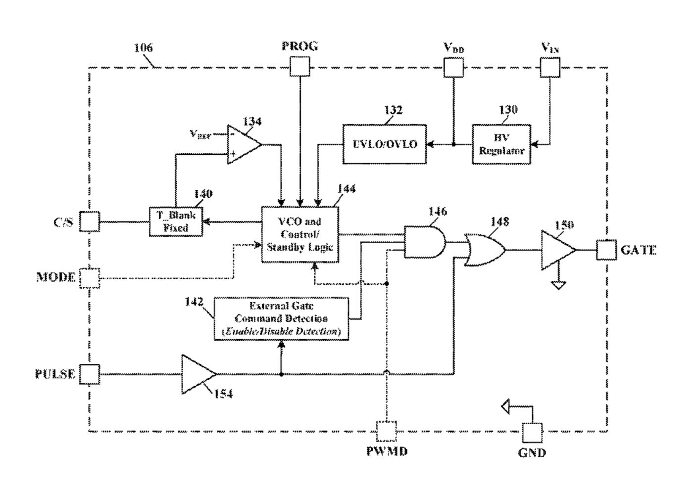
ondary-side controller may send an enable code command to the start-up controller where it is detect to allow the start-up controller to operate in a normal fashion with the secondary side controller.
