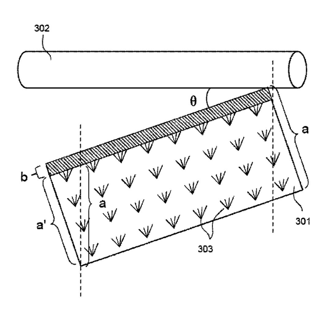
orientation process, the density of the rubbing loci can be increased without increasing the rubbing tuft density of existing rubbing cloth.
