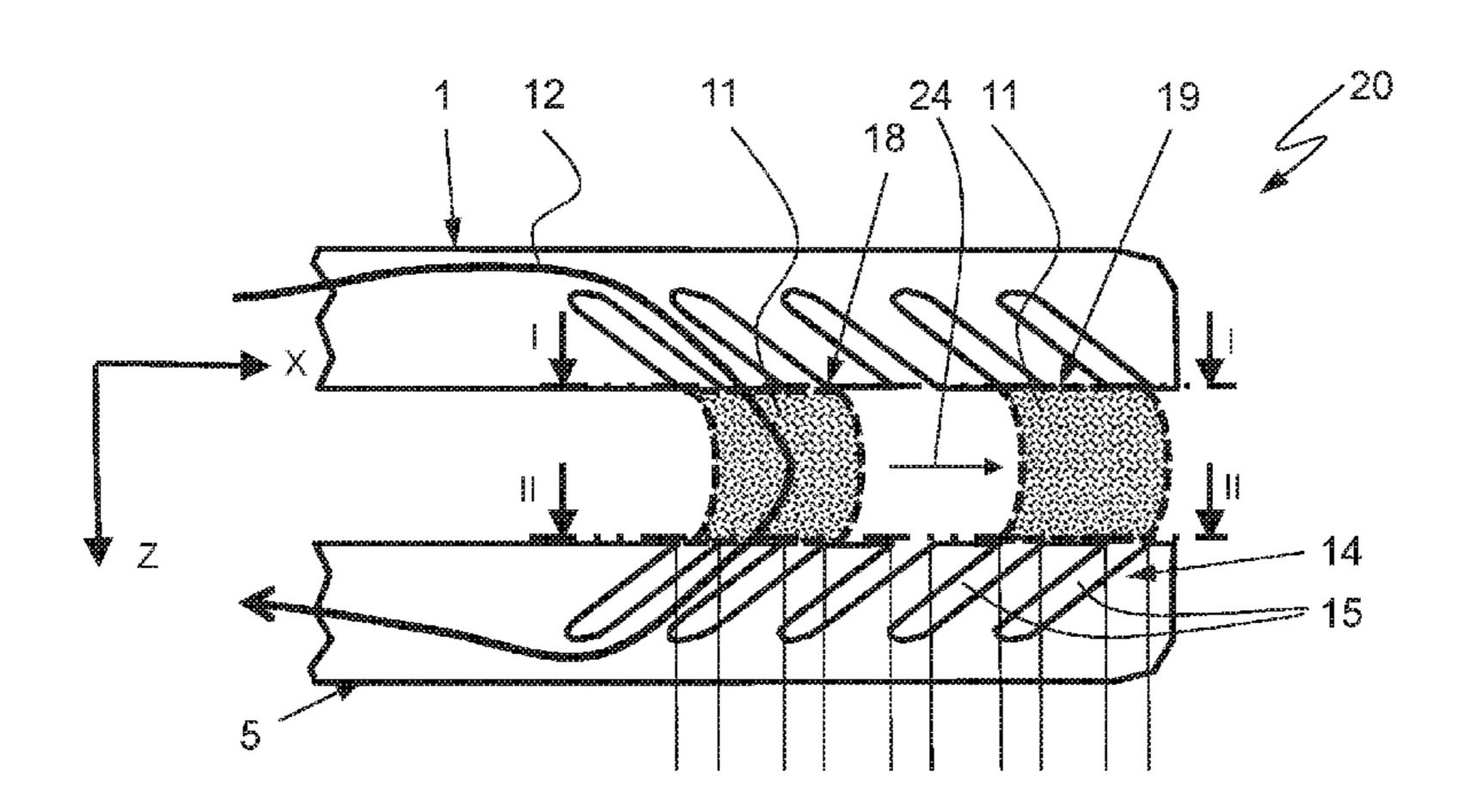
the first contact surface (4) after lifting the first contact surface (4) off the second contact surface (8) pushes said electric arc (11) in the direction of the apex of said first angle (17) from a first position (18) to a second position (19).
