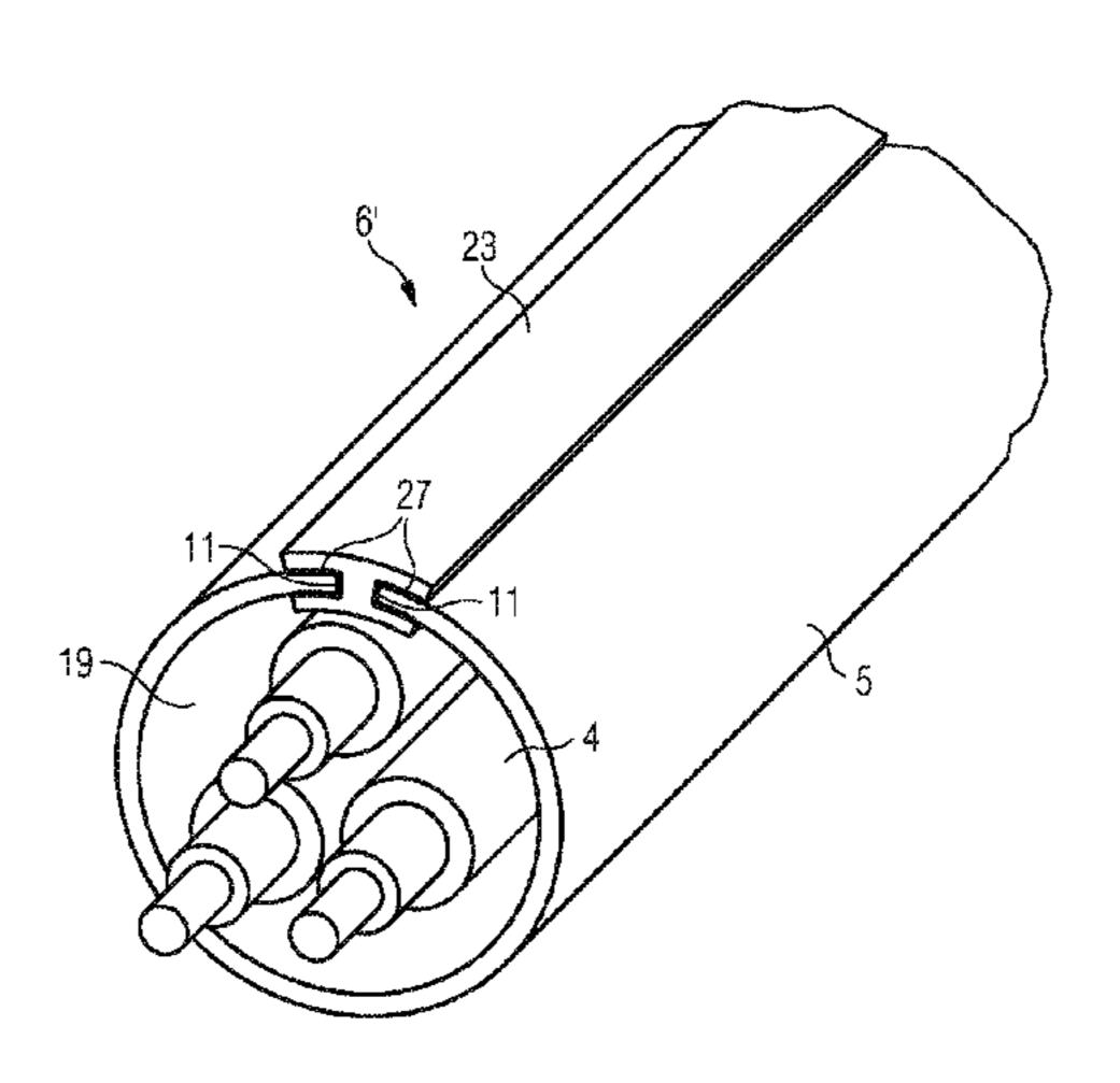
ductors into the cable-protecting pipe through the insertion opening in the open separating slit; and g) releasing the open separating slit.
