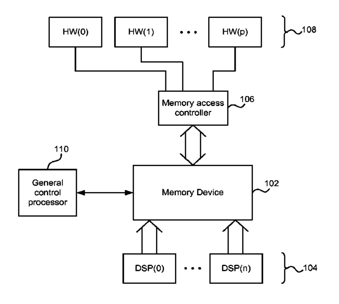
sive to this, control the memory access controller to enable a selected fixed function accelerator to read data from or write data to the memory device via its memory access channel.
