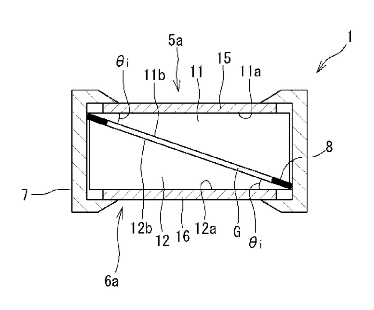
antireflective film which prevents reflection of normal incident infrared laser light, wherein  $\theta i$  is not smaller than a complementary angle  $\theta tB$  of a Brewster's angle  $\theta B$  of infrared laser light incident on a plate member and smaller than a critical angle  $\theta c$ , the inclined surfaces are opposed to each other via a gap, and the incident surface and the emitting surface are arranged in parallel to each other.
