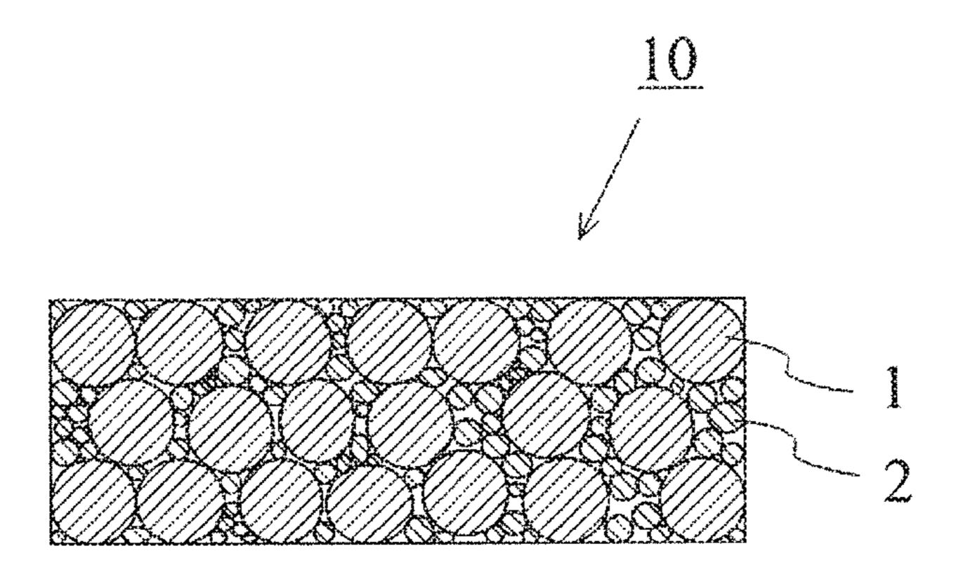
wherein the easily sinterable ceramic particles are interposed between the inorganic phosphor particles and the inorganic phosphor particles are bound together by the easily sinterable ceramic particles.
