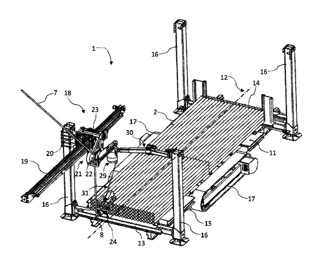
plane perpendicular to the elevated horizontal beam; and a drill rod and winch cable guiding means longitudinally movable along said boom.
