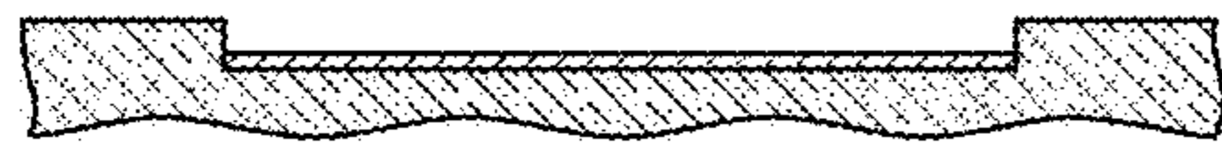
Recess & Shield Metal Layer
