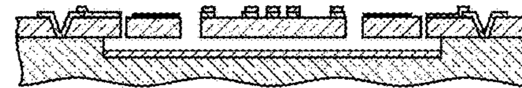
Isolation Platform and Isolation Suspension Pattern
