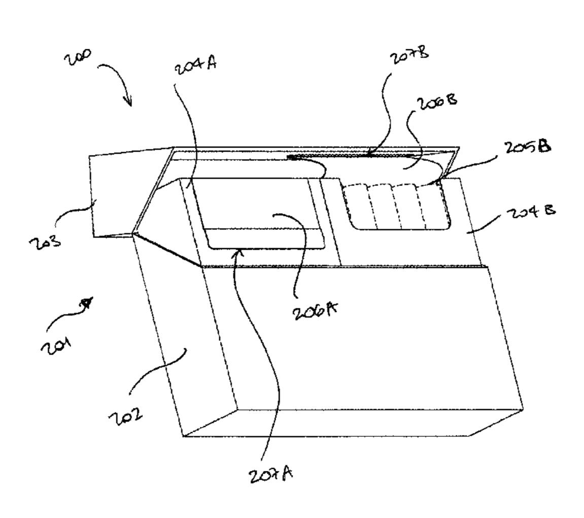
adhesive element, such that upon opening the lid the reclosable flap is lifted off the inner package to at least partly reveal the access opening.
