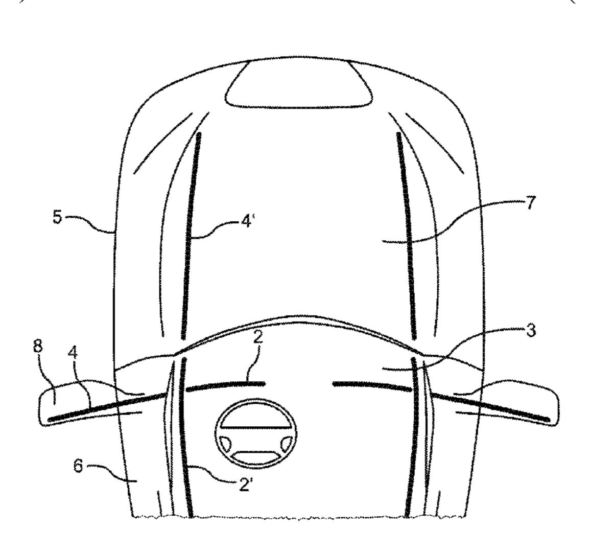
created by the second section (4, 4') of the illuminating fixture is radiated such that it is visible from a definable position relative to and outside of the vehicle (1).
