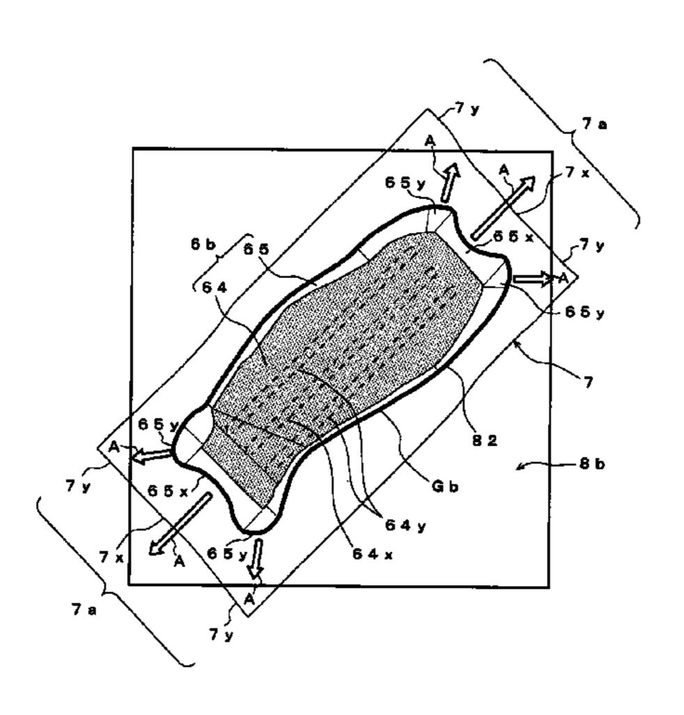
in the width direction. When the blank sheet is pressed against the fan blade mold, a center part in the width direction of the blank sheet at an end part in the longitudinal direction is pulled with a greater force than end parts in the width direction of the blank sheet at the end part in the longitudinal direction, thereby preventing occurrence of wrinkling.
