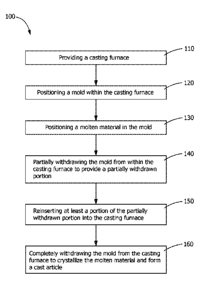
completely withdrawing of a mold from a casting furnace to form the cast article.
