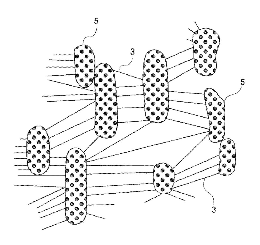
to 40% by weight of the total weight. The hot melt processable component is contained at equal to or more than 0.1% by weight but less than 20% by weight of the total weight. A drawn porous body includes a plurality of fibrils, and a plurality of knotted portions that are connected to each other by the fibrils.
