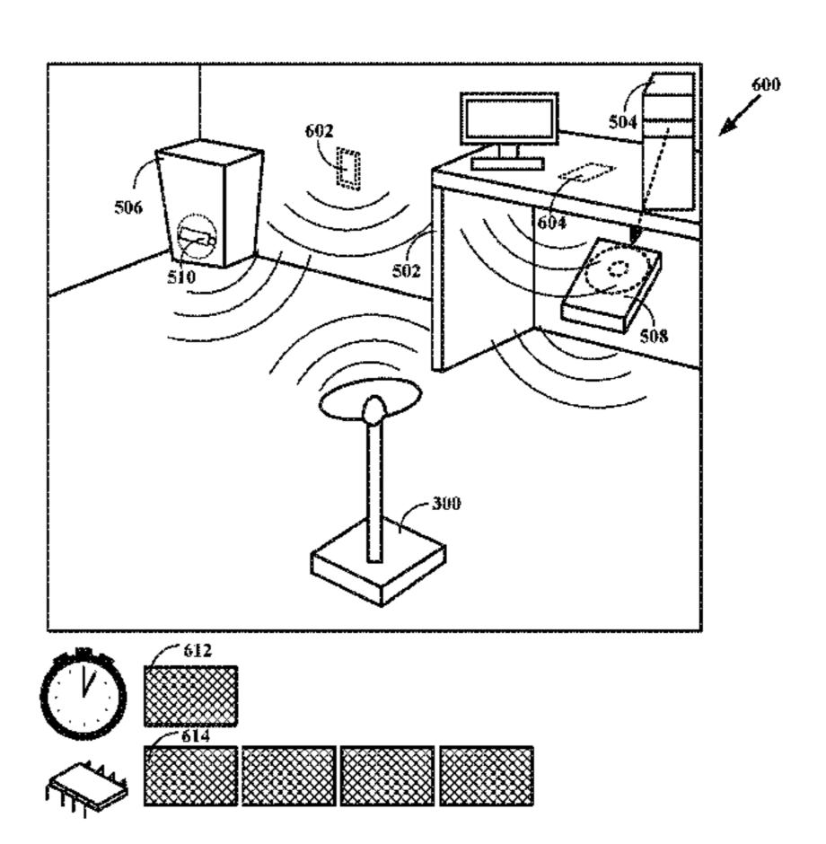
target device data is not affected. Embodiments can locate a hidden target device via the strength and directionality of the forced emissions. The apparatus is portable for use by military, intelligence, and security personnel.
