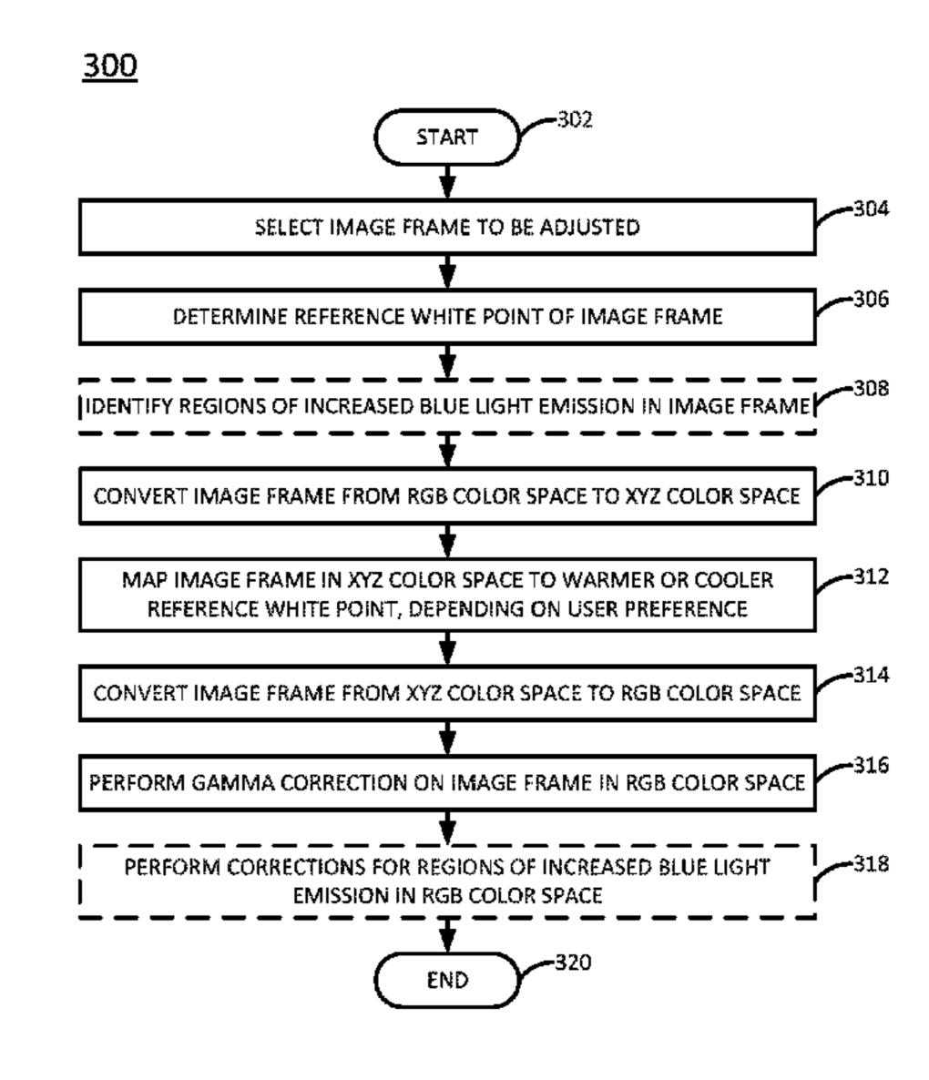
color temperature that scales the amount of blue light emitted by the display device. The subset of the plurality of image frames is then delivered to the display device, subsequent to the adjusting.
