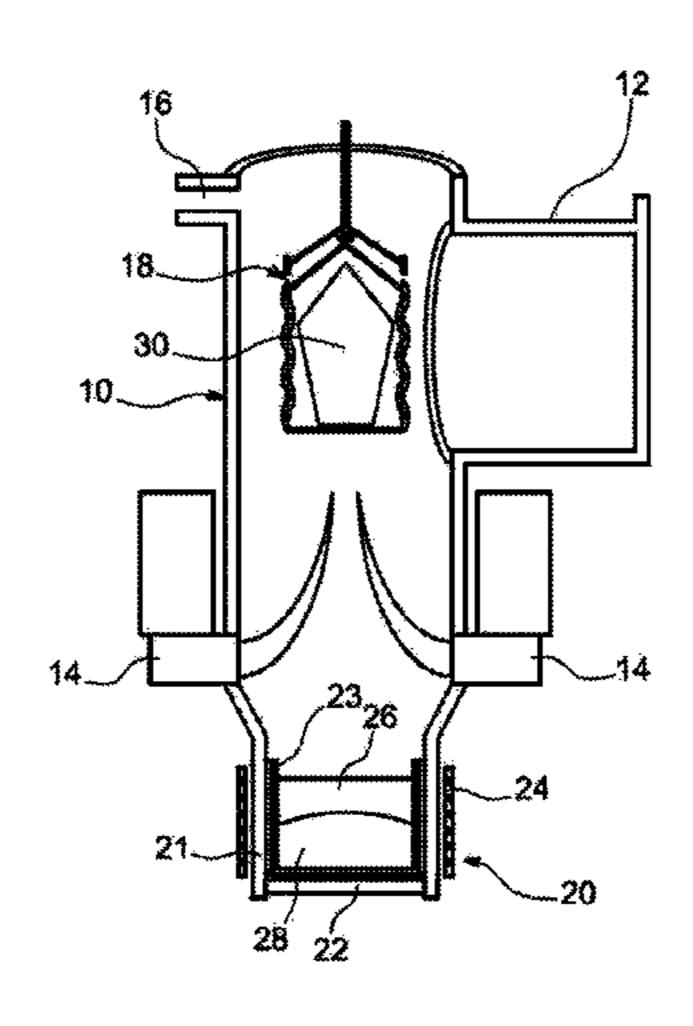
The furnace (20) can be dismantled, after a series of treatments of several baskets (18) of waste (30) for disassembling the crucible-forming container (23) from the furnace (20).
