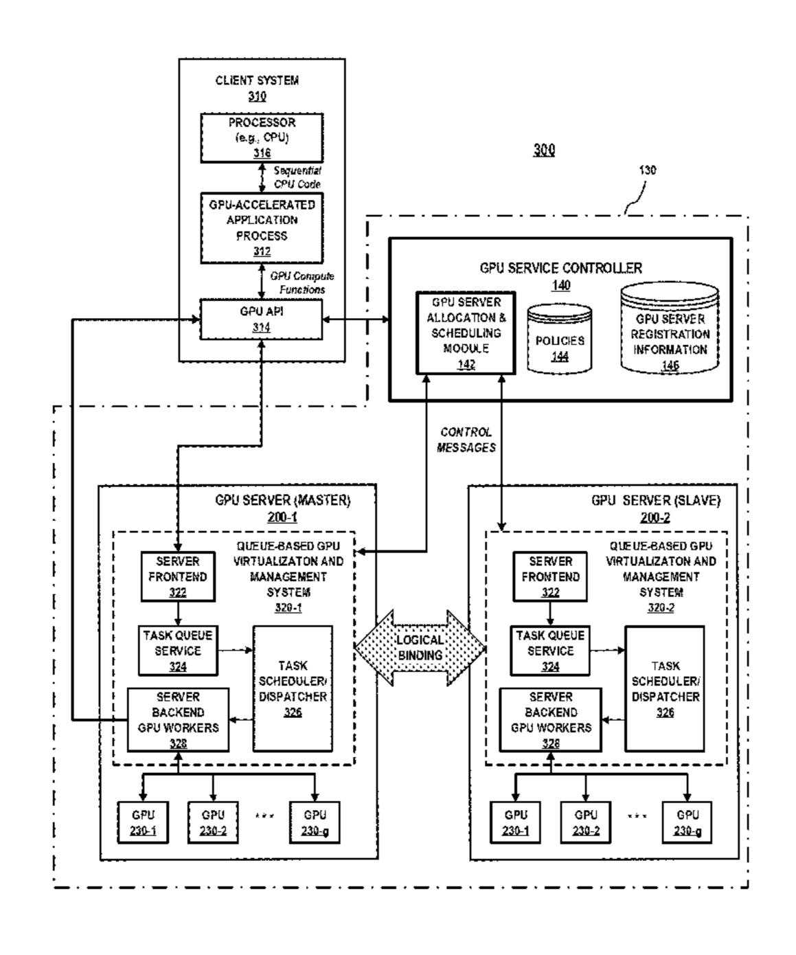
system, which is associated with the GPU processing tasks specified by the service request, processes the block of GPU program code using the GPU devices of the logically bound GPU servers, and returns processing results to the client system.
