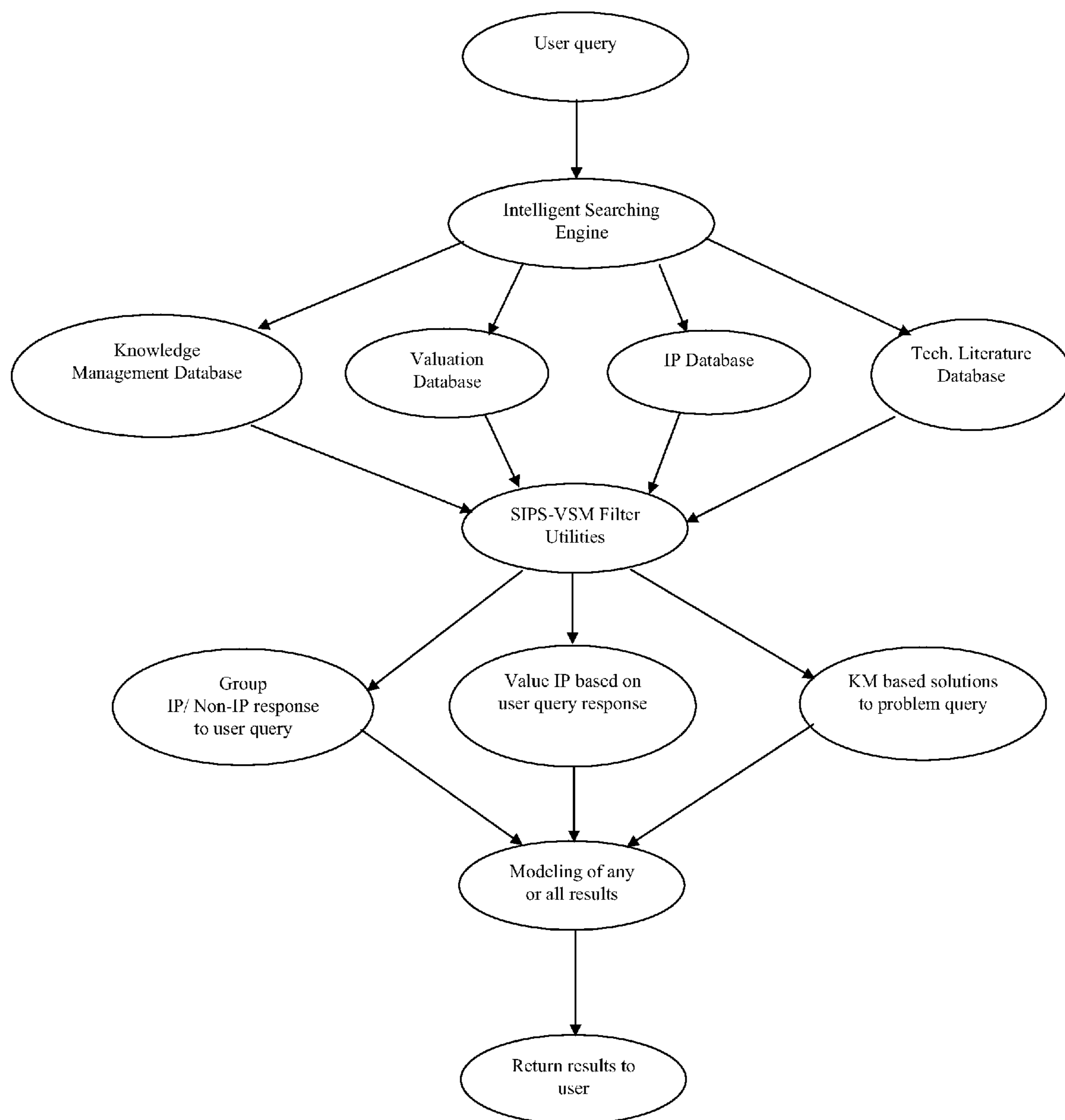
Figure 1. Programming logic scheme for SIPS-VSM Searching
