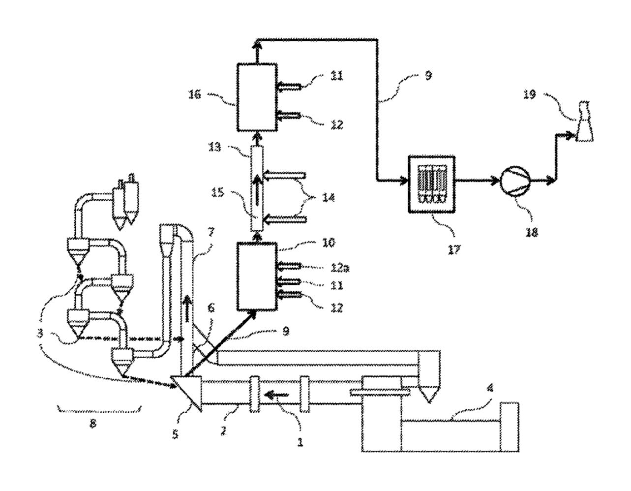
mixing chamber, in which the exhaust gas is cooled to between 800 and 950 degrees C., then the exhaust gas is guided through a reaction pipeline segment, wherein the dwell time is between 0.5 and 3 seconds and ammonia, aqueous ammonia solution, or ammonia-releasing substances are injected for denitrification. Then the exhaust gas is guided into a second mixing chamber, in which the exhaust gas is cooled to between 150 250 degrees C. Then the exhaust gas is guided to a filter for dust removal.
