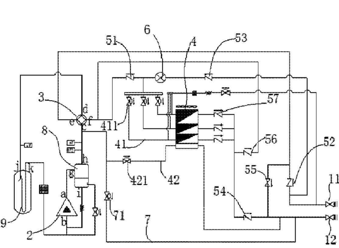
one-way valves, wherein each one-way valve has a circulation end and a stop end, and each one-way valve is opened only in one direction from the circulation end to the stop end; a throttling element; and a gas-liquid separator.
