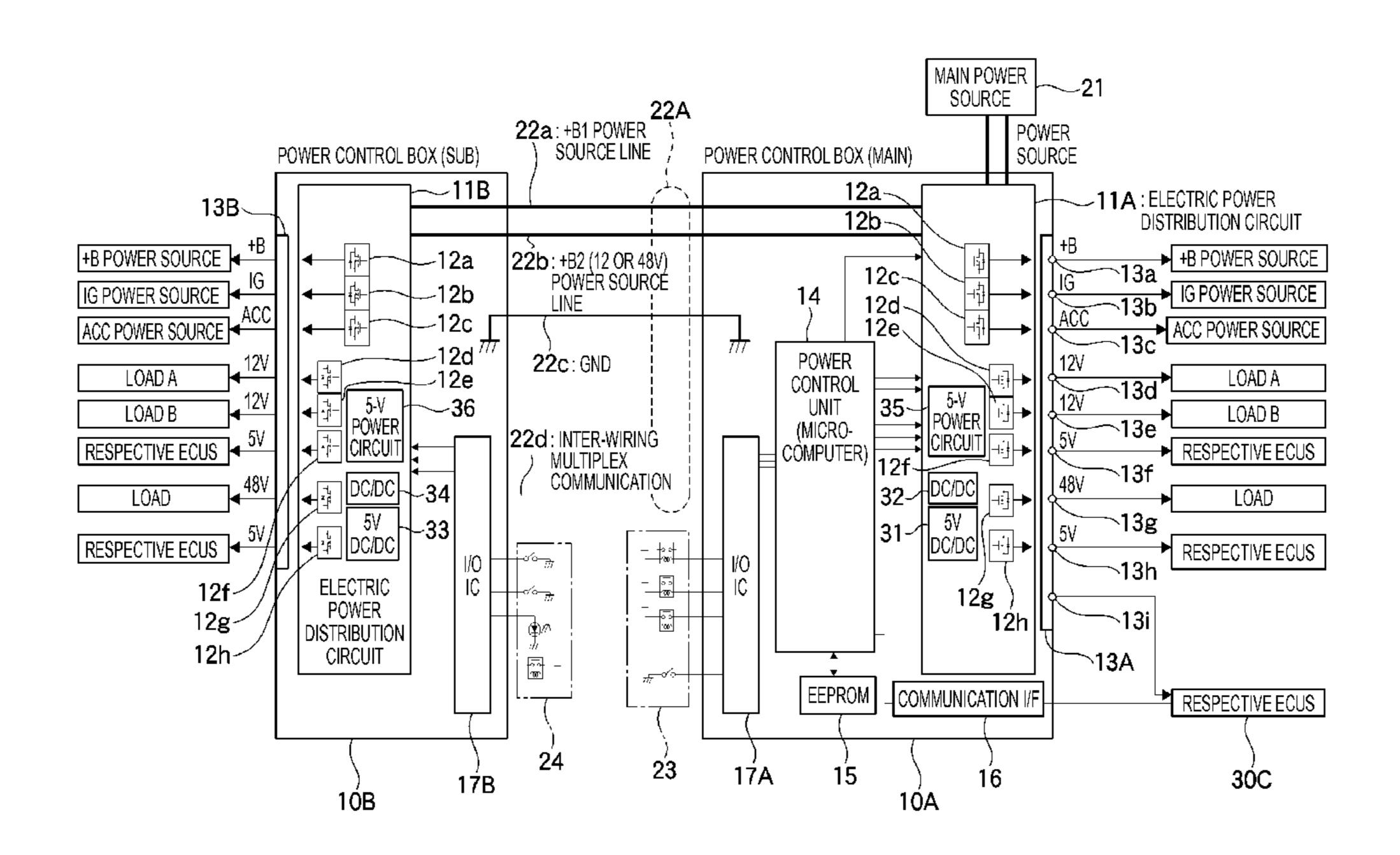
determined. The power control unit controls distribution of electric power to the respective ones of the plurality of loads or electronic control units by the power distribution unit, on the basis of the operation specifications determined in the customized information.
