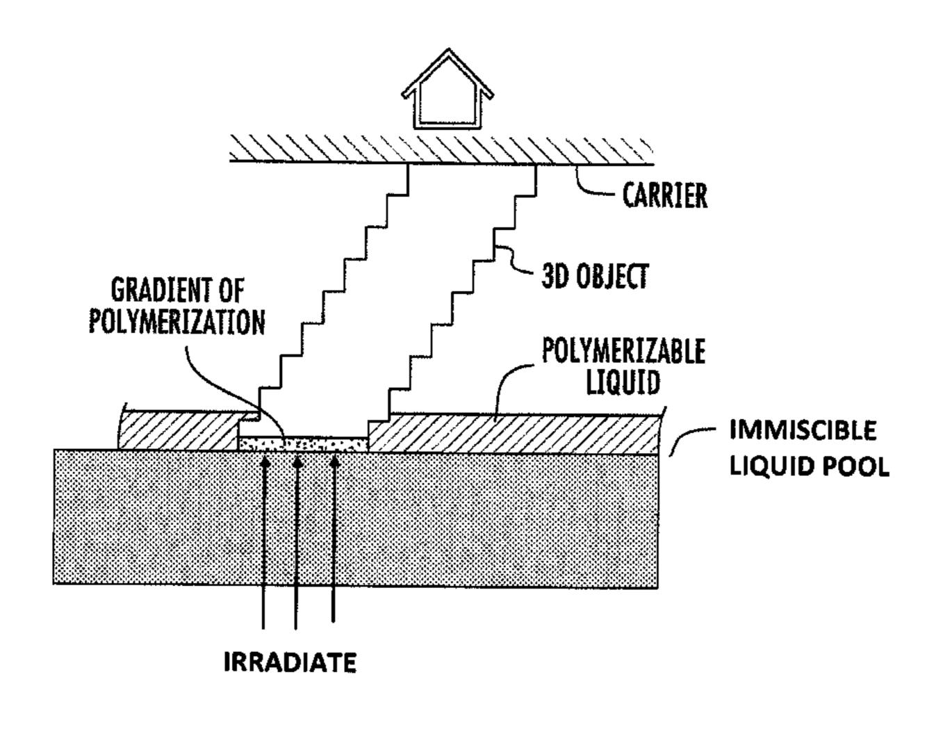
the liquid build surface to form the three-dimensional object comprised of the solid polymer from the polymerizable liquid. Optionally, but in some embodiments preferably, the method is carried out while also continuously maintaining a gradient of polymerization zone between the liquid build surface and the solid polymer and in contact with each thereof, the gradient of polymerization zone comprising the polymerizable liquid in partially cured form.
