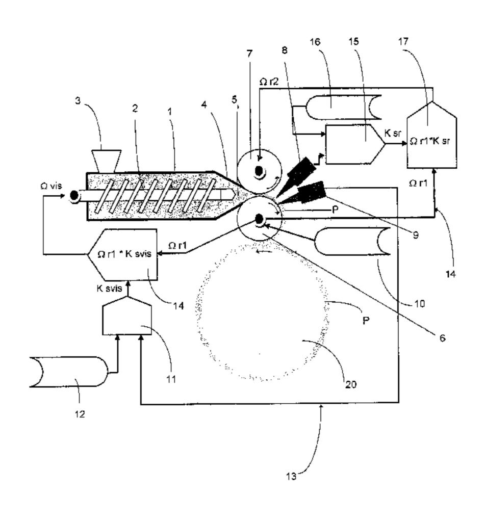
can regulate the speed of rotation of the screw depending on the width of the strip, and a second control means can regulate the speed of rotation of the second roll depending on the thickness of the strip.
