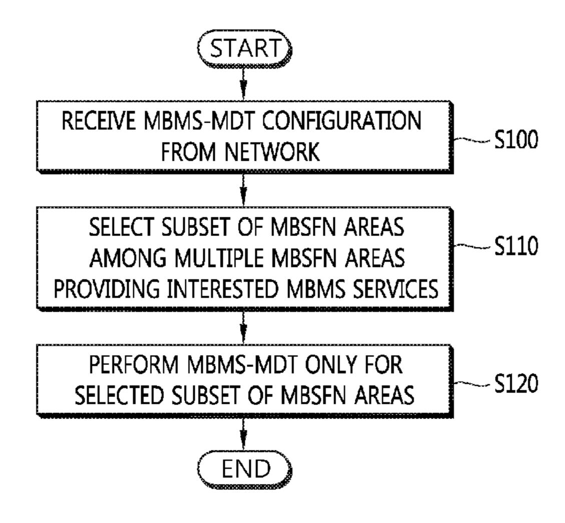
work, a user equipment (UE) selects a subset of multicast broadcast single frequency network (MBSFN) areas among multiple MBSFN areas providing interested MBMS services, and performs MBMS-MDT only for the selected subset of MBSFN areas. The subset of MBSFN areas may be selected based on priorities of the multiple MBSFN areas.
