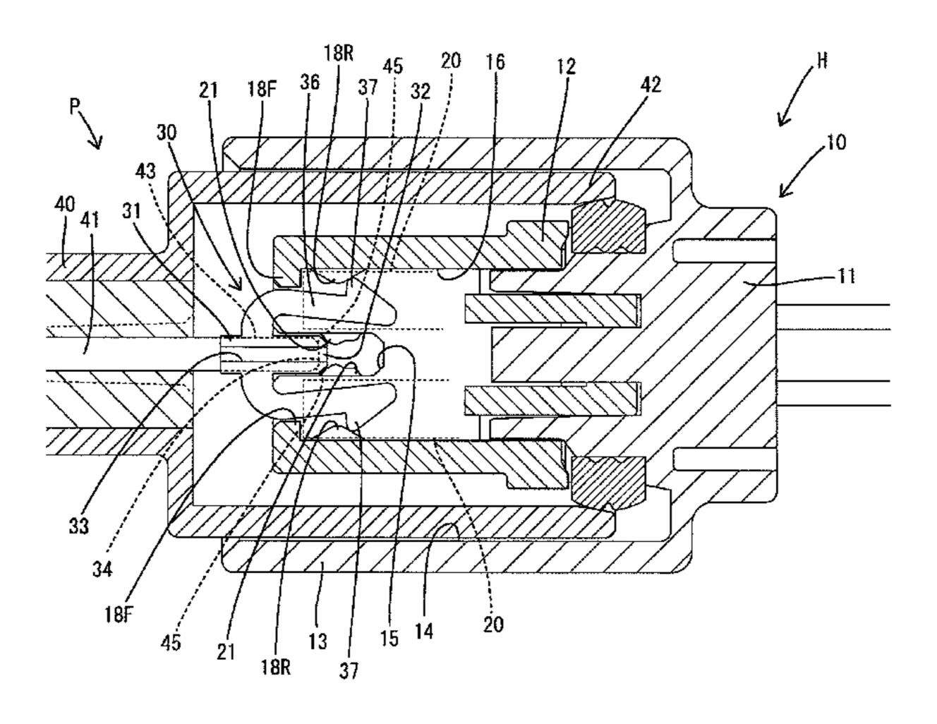
with the circuit board (41) in a withdrawing direction from the board accommodation space (15) by locking each other.
