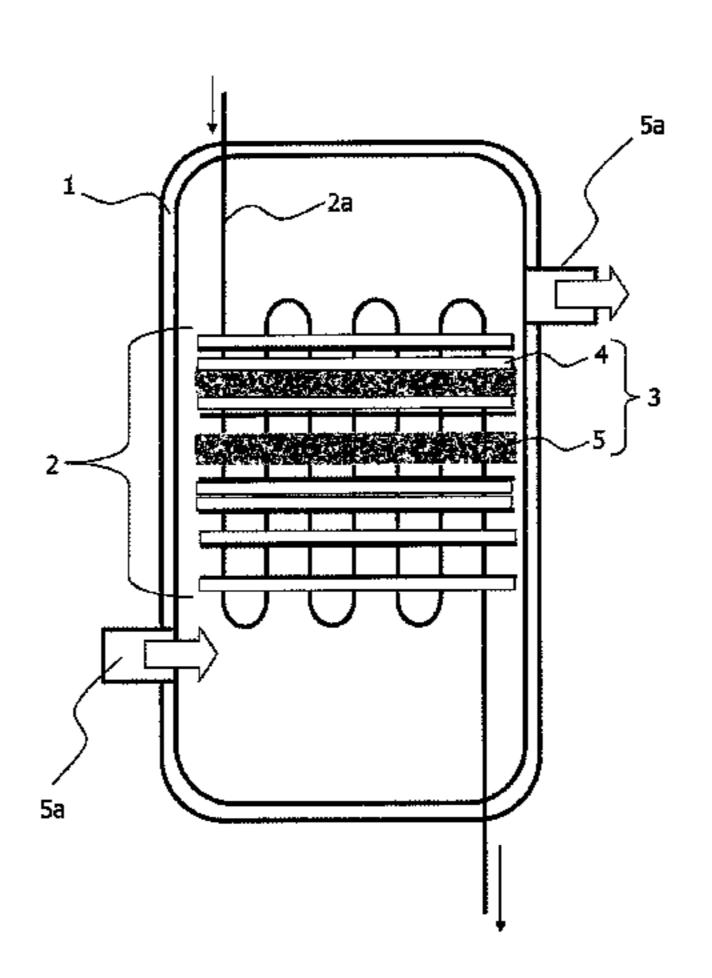
then evaporated from the heat transfer surface during the evaporation process. In terms of the apparatus, the heat transfer surface (2) is in the form of an in-situ store for a condensate film (6) of the working medium which covers the heat transfer surface and does not drip off and remains on the heat transfer surface during the condensation process and evaporates during the evaporation process.
