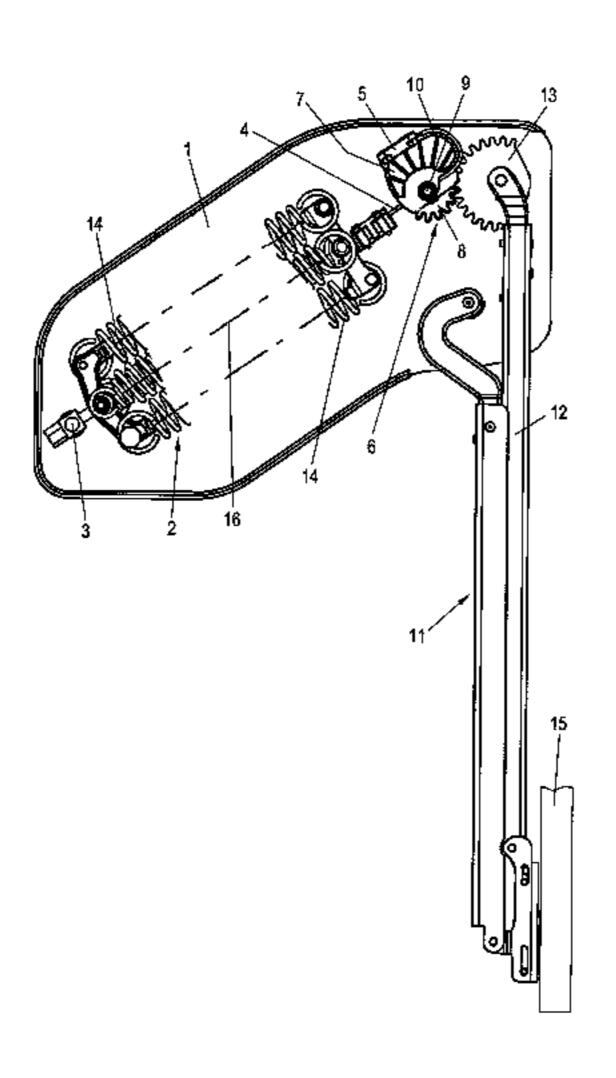
clamped, and in the other end position is unclamped relative thereto, and wherein the cam disc has a control contour with varying radius of curvature, on which cam disc the energy accumulator is held.
