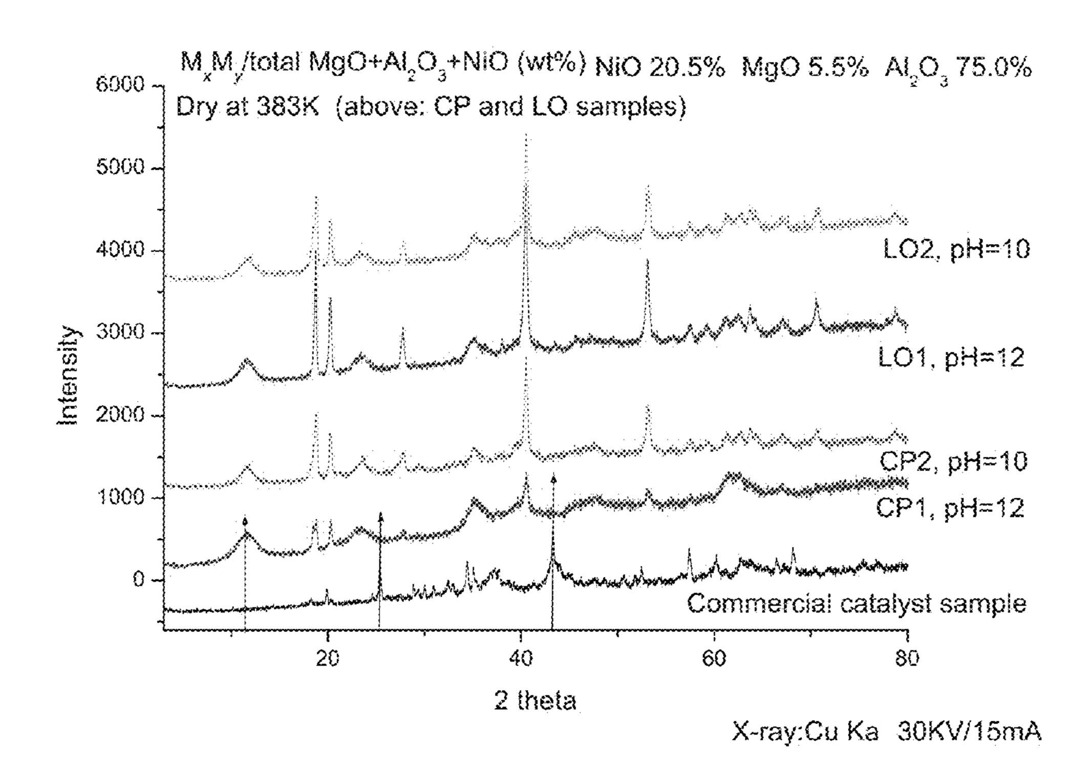
PXRD (homemade samples and Com. Sample)
