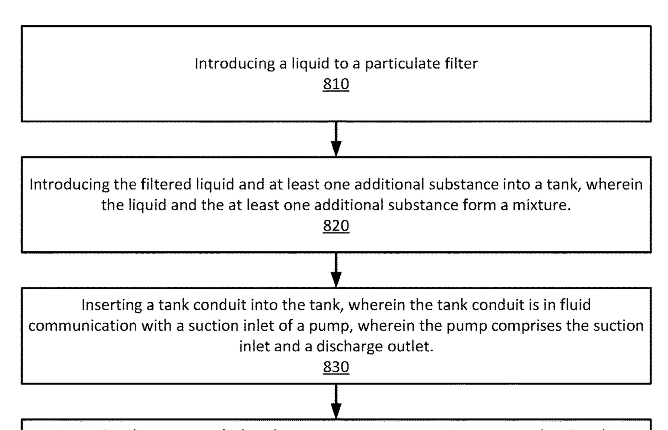
Operating the pump such that the pump creates a negative pressure drawing the mixture into the pump through the suction inlet and wherein the pump creates a positive pressure expelling the mixture out of the pump through the discharge outlet. 840
