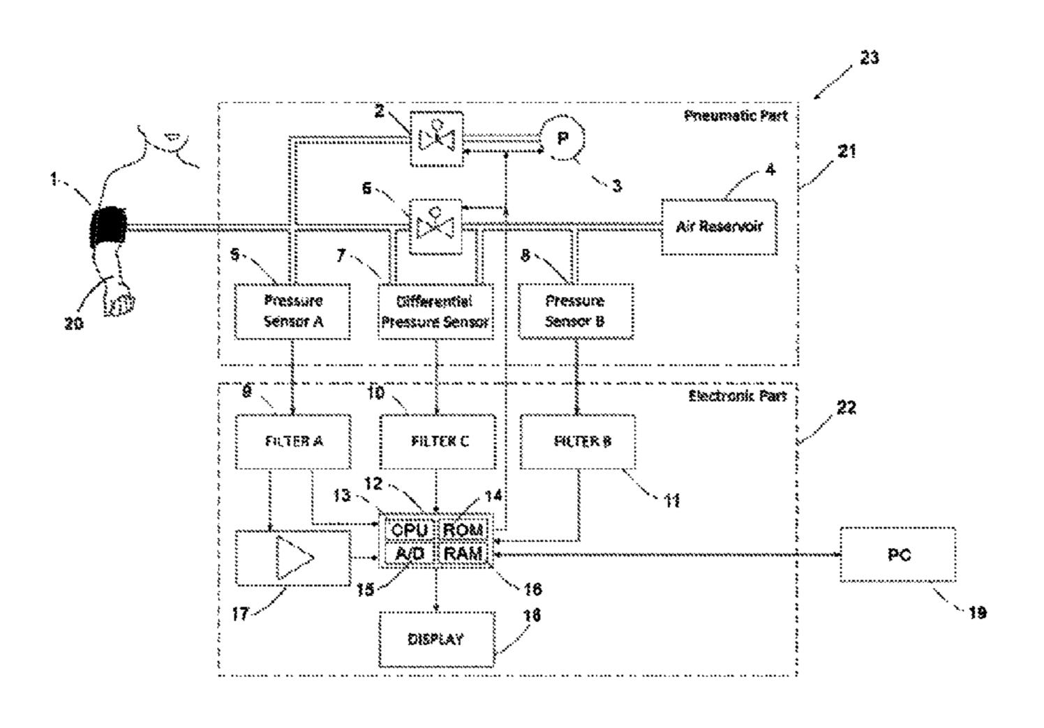
algorithm in the microprocessor, according to signals from the pressure sensor A further controls the course of cuff pressurization, controls the control valve, and finally determines the closing and opening of the closing valve. A microprocessor further controls a display and the data may be transmitted to the PC.
