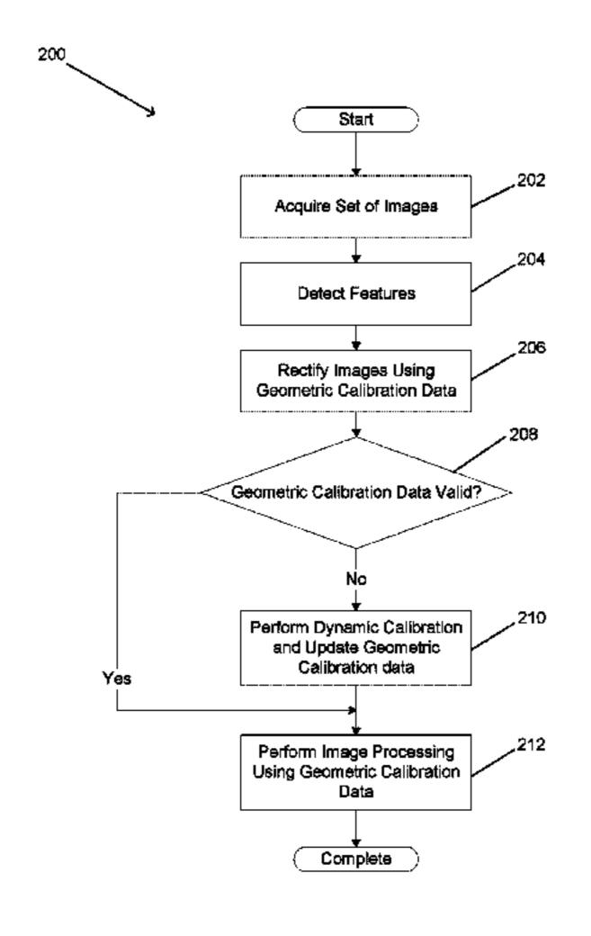
geometric calibration from amongst a number of different sets of geometric calibration data that is the best fit for the current geometry of the camera array.
