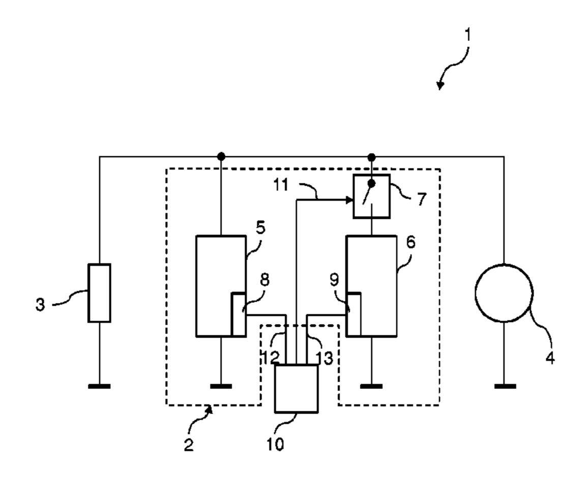
previous state of charge determination process in parallel with the state of charge and expressing the quality of the balancing exceeds a predefined threshold value. When the two criteria are fulfilled, the quiescent voltage measurement device for determining the state of charge of at least the first energy store is activated.
