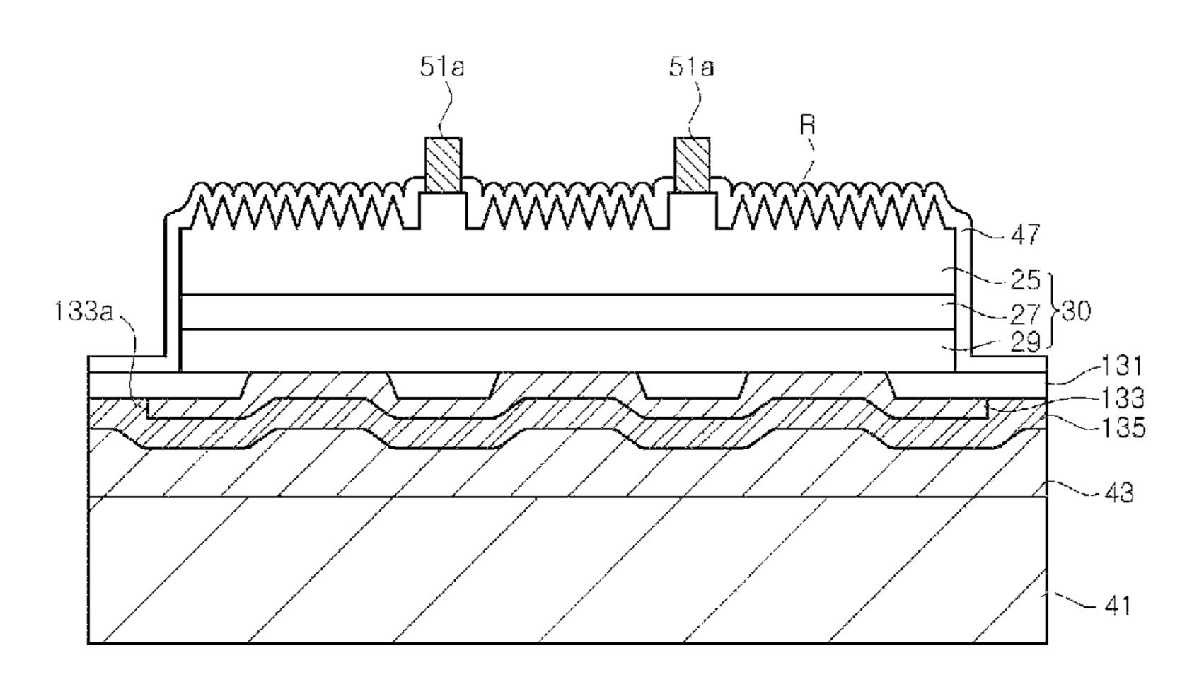
covers a surface region of the p-type semiconductor layer under the contact region of the electrode extension, and a second insulating layer interposed between the first electrode pad and the semiconductor stack.
