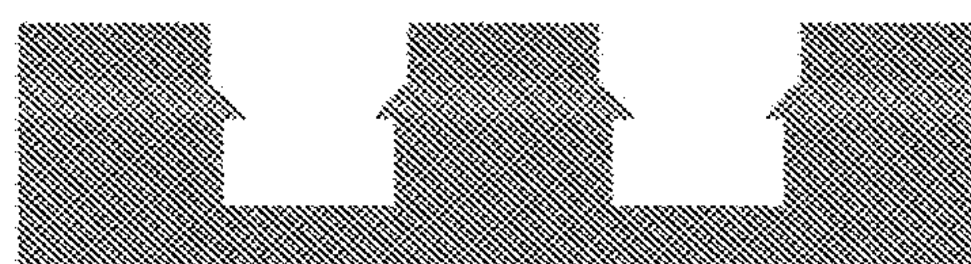
DRIE of CNT cavities in Si
