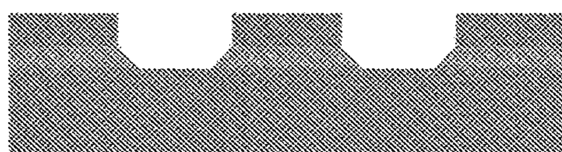
SiO 2 etch in BOE solution
