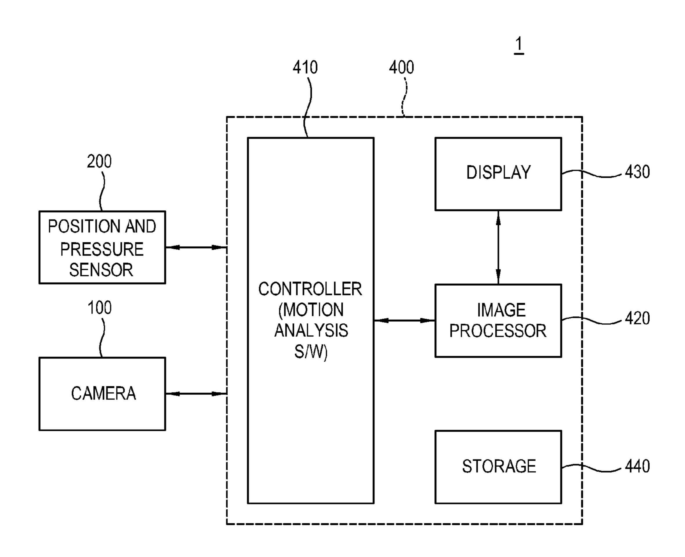
DISPLAY MOTION ANALYSIS COMPUTER (S/W) STORAGE POSITION AND PRESSURE SENSOR CAMERA 100
