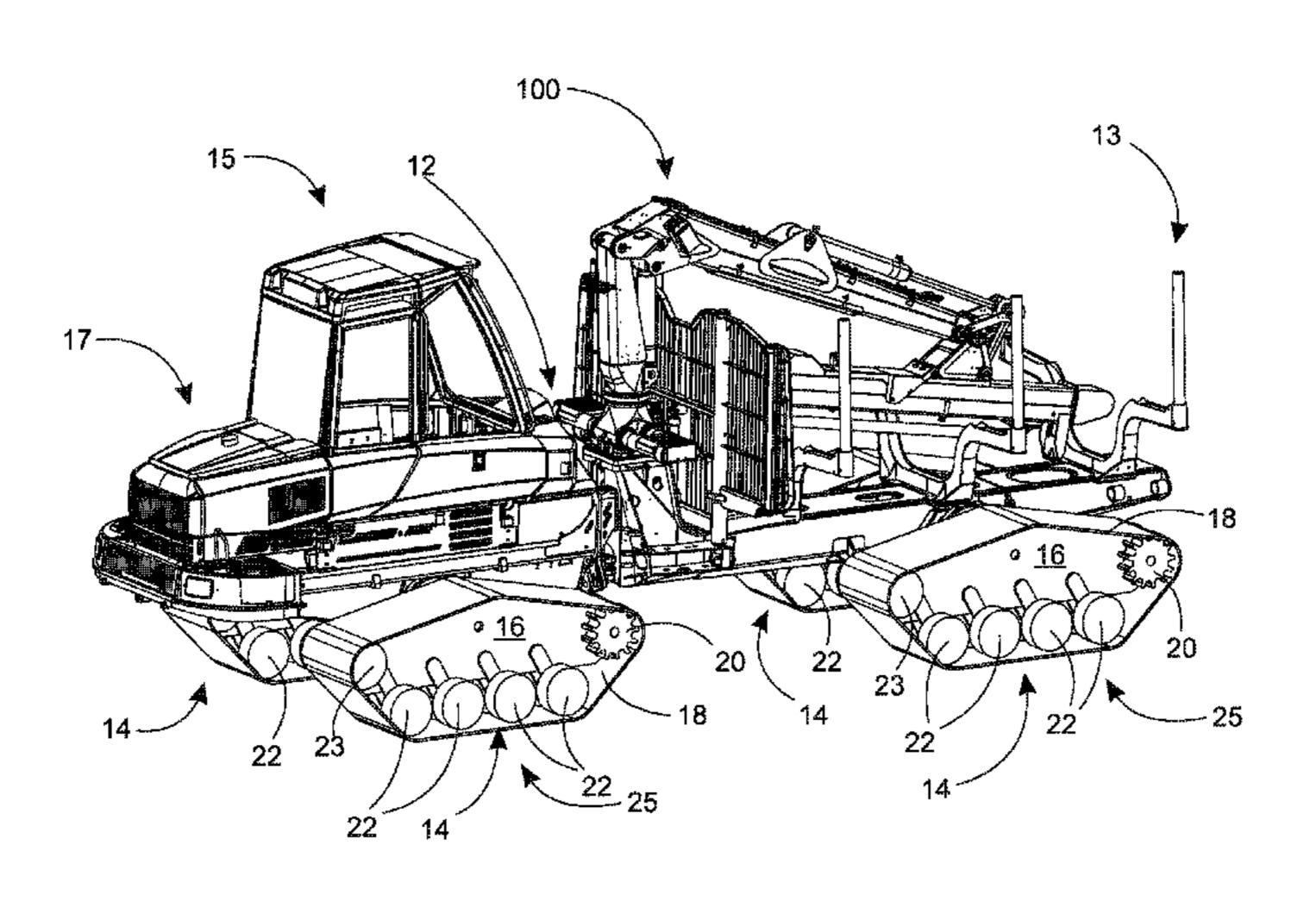
crawler-track unit. A shaft mounted in bearings on the crawler-track frame pivots the drive wheel to the crawler-track frame at a distance from the drive shaft. A power-transmission is fitted between the shaft and the drive shaft to transmit power from the drive shaft to the drive wheel.
