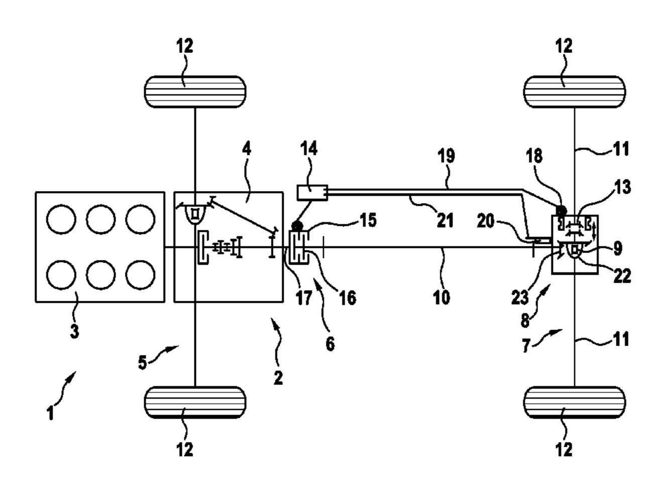
all-wheel drive is disabled, the rotational speed (n) of at least one of the uncoupled components is measured in a time interval, and an angular acceleration of the uncoupled components is determined therefrom.
