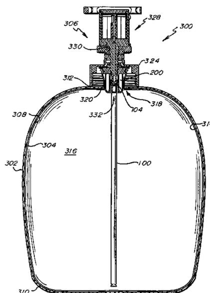
lower neck portion is configured to extend into the interior of the container.
