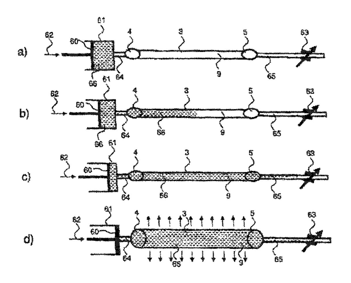
state of charge and the thereby resulting changes in the length of the series arrangement.
